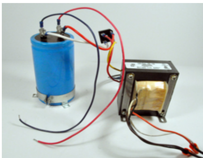
Fig: A typical AC-DC adapter using a transformer, a bridge rectifier and a smoothing capacitor
